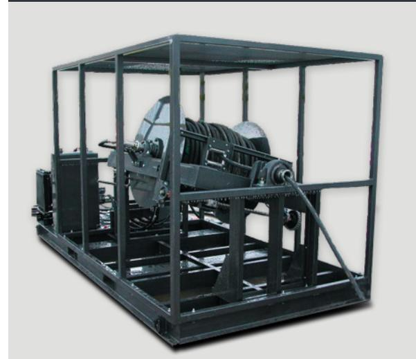
NLB's high-capacity hydraulically-driven Roto-Reel® hose reel spools a hose at 60 feet per minute and feeds it out at 40 feet per minute.
